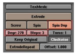
Switch to front view and go to the edit buttons with F9. Set the highlited buttons. We are going to duplicate the fins with the 'SpinDup' command. The 3D cursor must be at the center of the body.
