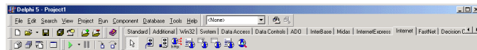
Figure 1: The Internet page of Delphi’s component palette, hosting the socket and HTML producer components.
